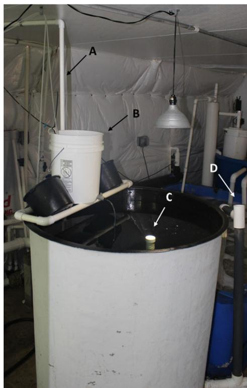
FIGURE 1. Photograph depicting the configuration of the larval rearing tank used for culture of Pacific blue tang larvae. (A) Water inflow pipe, (B) feed bucket, (C) screened internal stand pipe, and (D) external standpipe. [Colour figure can be viewed at [wileyonlinelibrary.com](http://wileyonlinelibrary.com)].
